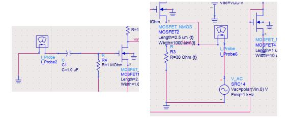
With these changes, the relationship between the test voltage and measured current was simulated to generate the plot below. Again, the axes are inverted due to the limitations of Keysight ADS, so the output impedance was measured to be  $16.1\,\Omega$ .
