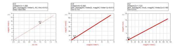
The voltage gain of the entire amplifier was likewise measured in the simulation, with a gain of 10.65, or 20.55 dB:
