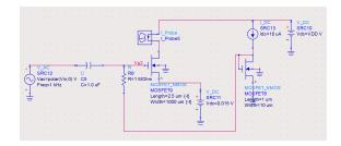
The input signal and biasing network were left unchanged, but the resistor at the drain/source was replaced with a constant DC voltage source, as fluctuations in the biasing conditions due to the voltage drop of the resistor would interfere with measurements of transconductance. The voltages of the sources were determined by a DC analysis of the original circuit in operating condition. The results of these tests are shown below:
