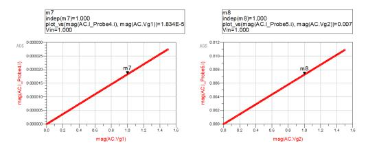
From this testing setup, the transconductance of the first two MOSFETs was determined to be  $g_m = 18.3 \,\mu\text{S}$ . The value for the third MOSFET was  $g_m = 7 \,\text{mS}$ .
